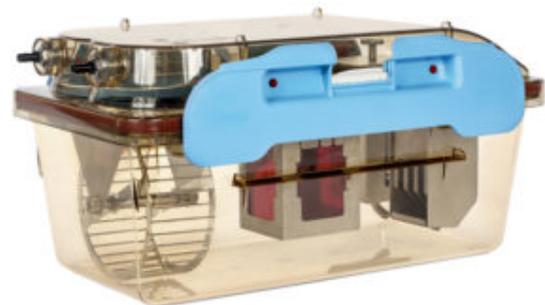
Each cage is connected to a flow regulator and gas analyser to measure oxygen consumption and carbon dioxide production.
