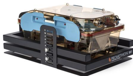
Cages are situated within an X, Y, Z beam-break matrix which detects activity.
