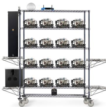
The Promethion Metabolic System from Sable (Nevada, USA) is a comprehensive lab animal metabolic activity monitoring system. It incorporates sub-systems for open circuit gas exchange calorimetry, movement, body mass, feeding, drinking, and running wheel activity in an environmental chamber.
